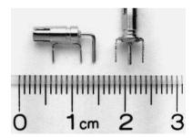
The HP PC board mini-probe sockets are ideal for reliable, stable, and convenient connection between the 10400 family probe tip and the circuit under test. The HP 1250-2427 horizontal PC board mini-probe replaces HP 1250-1737. The HP 1250-2428 vertical PC board mini-probe socket replaces HP 1250-1918.
